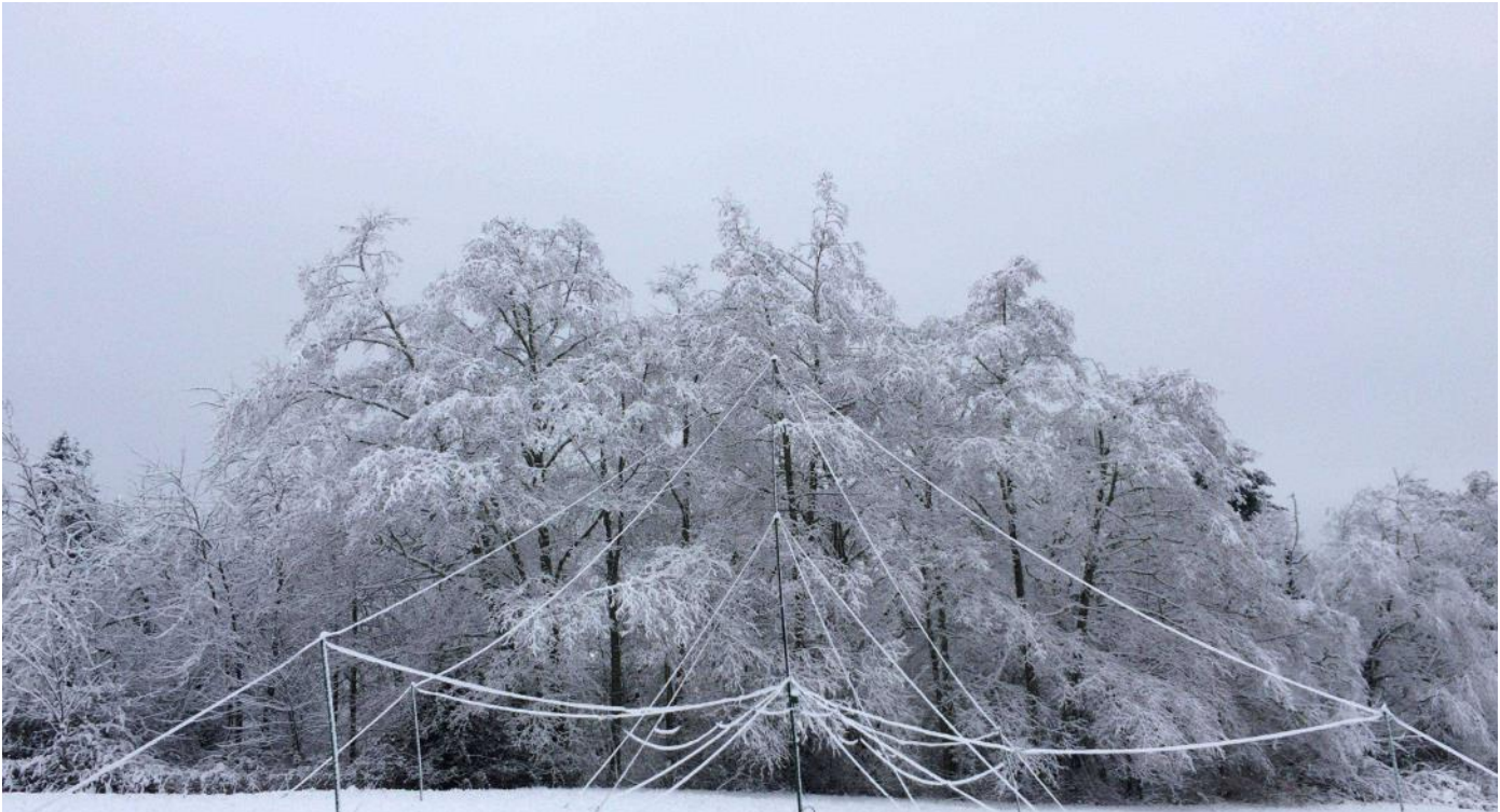
This is Mark, K6UFO's, SAL-30 at his Washington State QTH. Mark notes "Refurb needed every spring after weather, snow, wind, deer running through the field." This is the older Array Solutions model with fiberglass mast.
