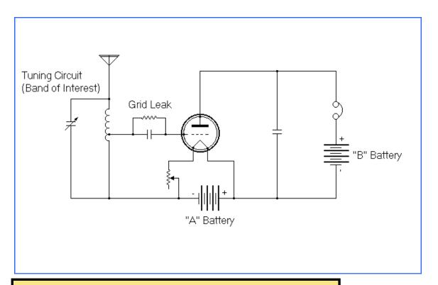
This is a basic one-tube radio receiver. The triode tube is a refinement of the DeForest Audion. Back in the day, one needed to draw schematics like this (or something similar) during the General Class Amateur examination. Good luck finding a "B" battery today.
