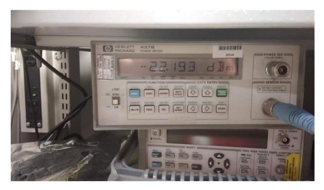
All steps are disengaged here, and signal generator is set to -6 dBm a change of 106 dB from previous picture.
