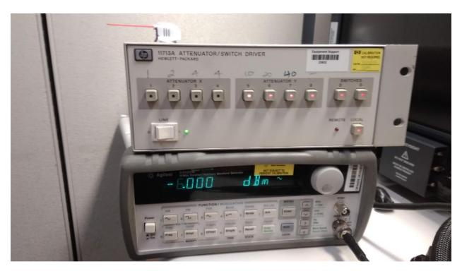
Power out is now -20.119 dBm with in at -6 dBm. Only about 2 dB of change over 106 dB of change on the input. The magic func(on of an AGC.
