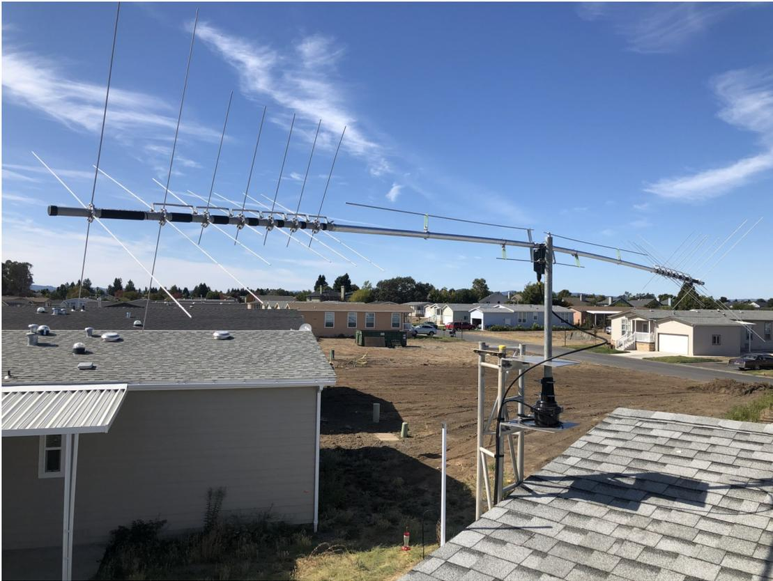
The finished product in place revealing the rotatable dipole and a set of 2 meter elements
