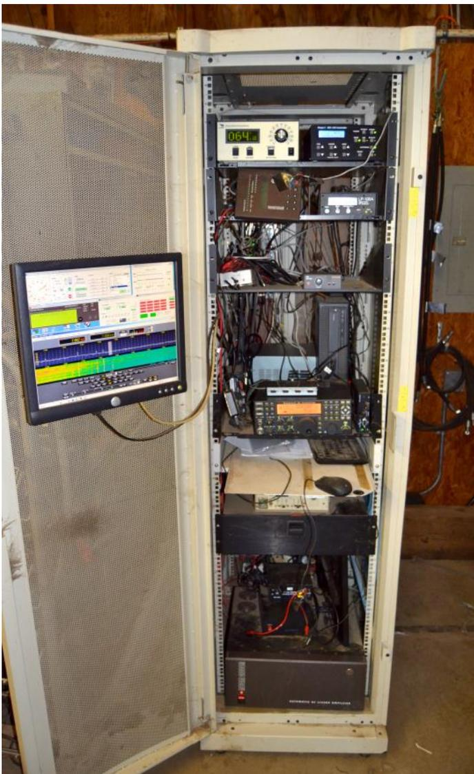
To the left is the N6IE shack-in-a-closet where, from top to bottom, you can see a Green Heron rotor control, SteppIR SDA-100 controller, Elecraft K-3, and ACOM 2000. Toward the rear of the closet is the PC that controls the operation.
