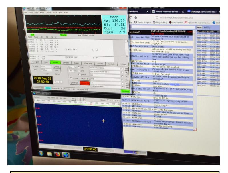
Above, a JT-65 EME QSO between W6XU and W7GJ Montana) using WSJT software. The faint white vertical trace against the blue background is the W7GJ signal. The Moon is between 225,623 and 252,088 miles from
